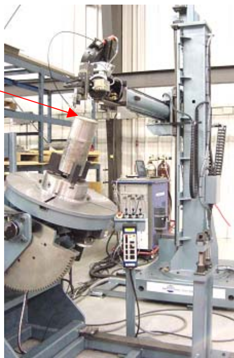
Inconel buttering of stainless steel tube ends
