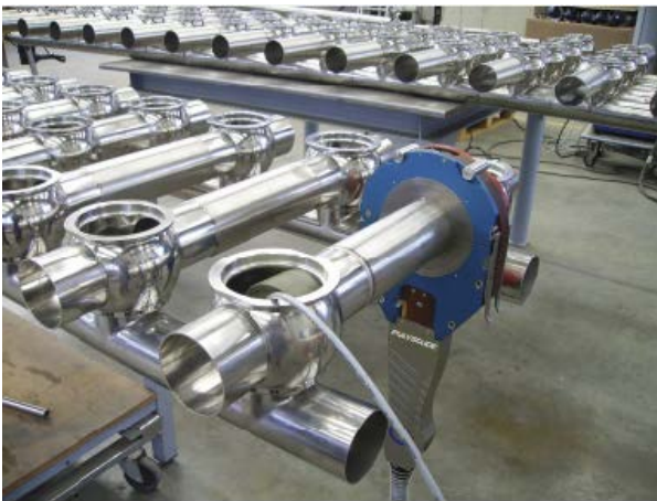
Fig.6: Orbital welding equipment on stainless steel tube with backing gas for the oxidation-free welds (photo Polysoude)
