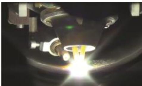
Fig.2 Detail of a working TIG<sup>er</sup> torch
