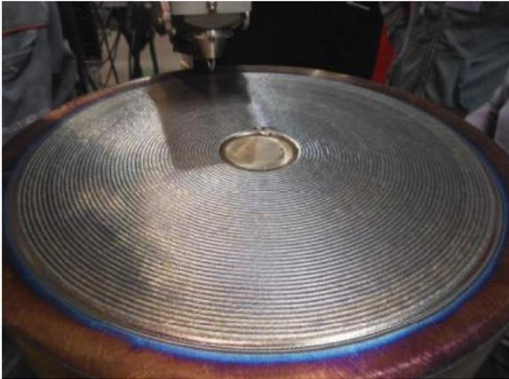
Fig.6 Realisation of the cladded specimen with TIG<sup>er</sup> process (end of the first cladded layer)
