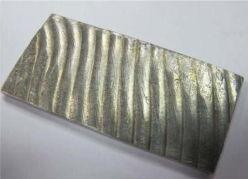
Fig.12 Sample subjected to corrosion tests ASTM G48 method A (after the test)
