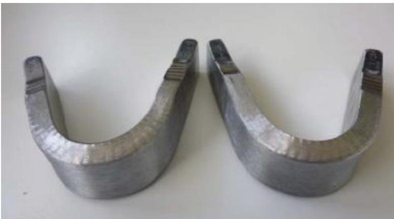
Fig.8 Samples subjected to bend tests according to ASME sec. IX, art II
