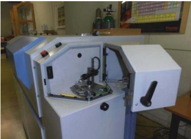
Fig.10 Optical emission spectrograph used for the chemical analysis of the clad layers
