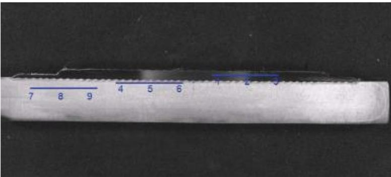
Fig.13 Macrograph of the specimen realized by TIG<sup>er</sup> process (highlights on hardness sampling areas)
