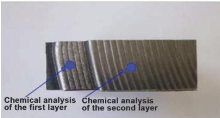
Fig.9 Specimen realised by TIG<sup>er</sup> process, highlighting areas of investigation for chemical analysis on the first and second layers.
