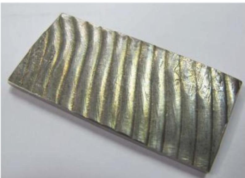
Fig.11 Sample subjected to corrosion tests ASTM G48 method A (before the test)
