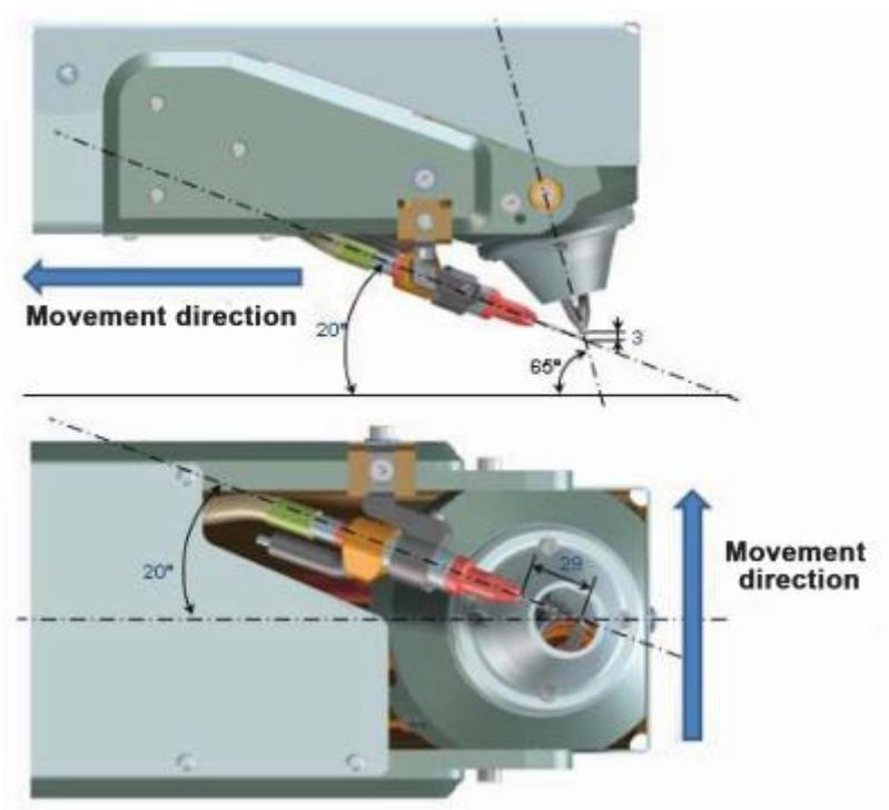
Fig.5 Configuration of a TIG<sup>er</sup> welding head
