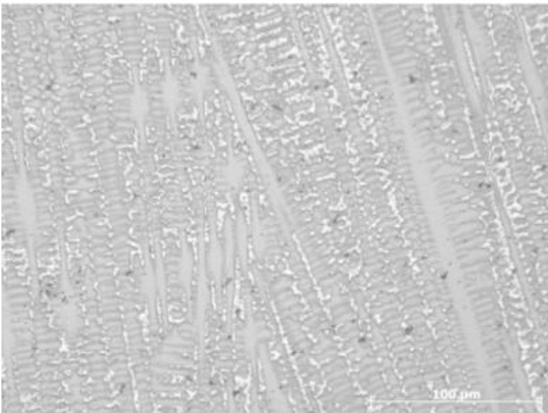
Fig.16 Dendritic structure of the molten zone
