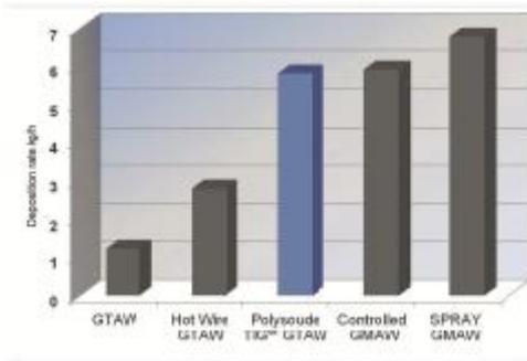
Fig.3 Deposit rate of TIG<sup>er</sup> technology in comparison with other processes (Source: Polysoude)
