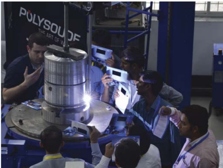
Fig.2: Weld overlay cladding demonstration
