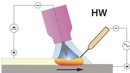
Fig.3: Hot wire TIG welding principle
