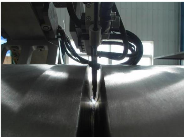
Fig.5: Narrow groove torch with its hot wire guide in a narrow gap joint
