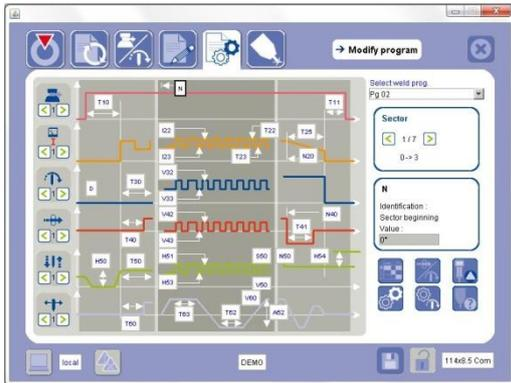
Fig.2: GUI presented on touchscreen to manage complete weld data and to use numerous auxiliary functions
