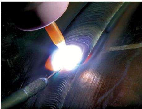
Fig.4: The shielding inert gas guarantees a perfect oxidation-free weld
