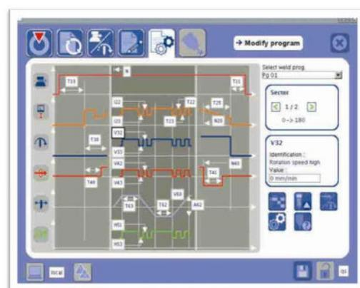
Fig. 4: Intelligent graphic user interface of the power source
