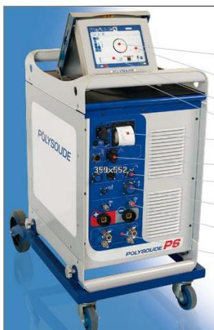
Fig. 3: Power source P6 for orbital TIG welding
