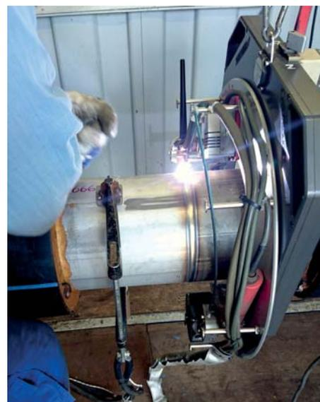
Figure 4. Orbital TIG welding head in action with pulsed current; during the phase of high intensity (pulse current) full penetration is achieved.
