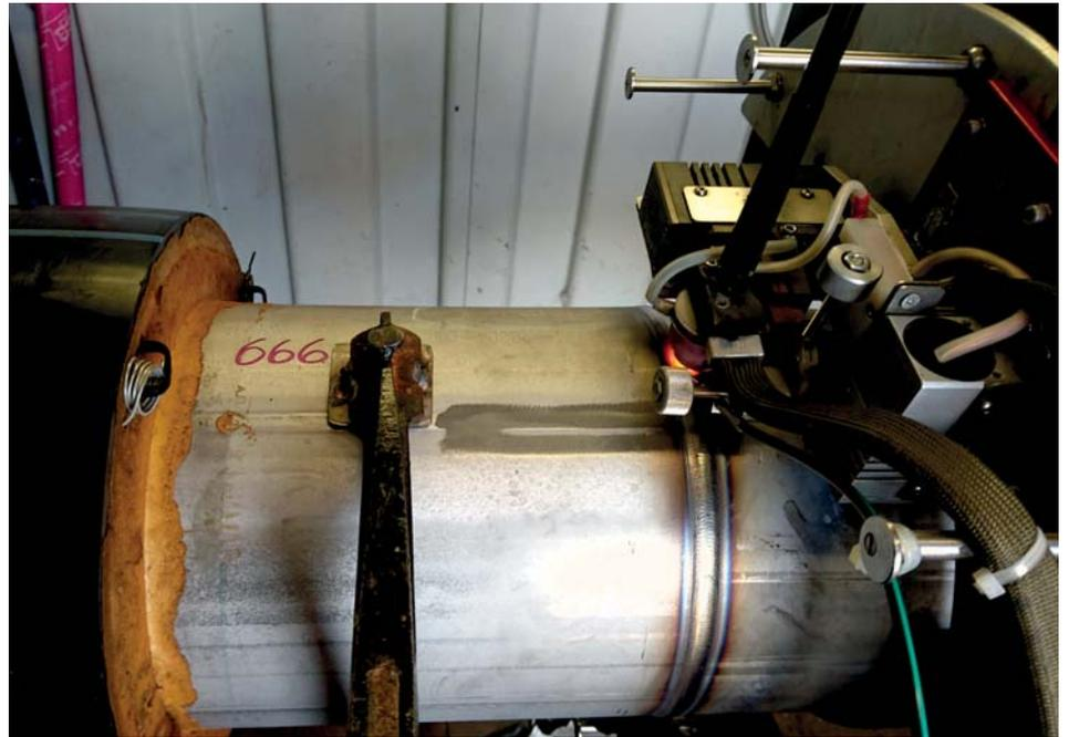
Figure 5. Orbital TIG welding with pulsed current; during the phase of low intensity (background current) the weld pool is stabilised.
