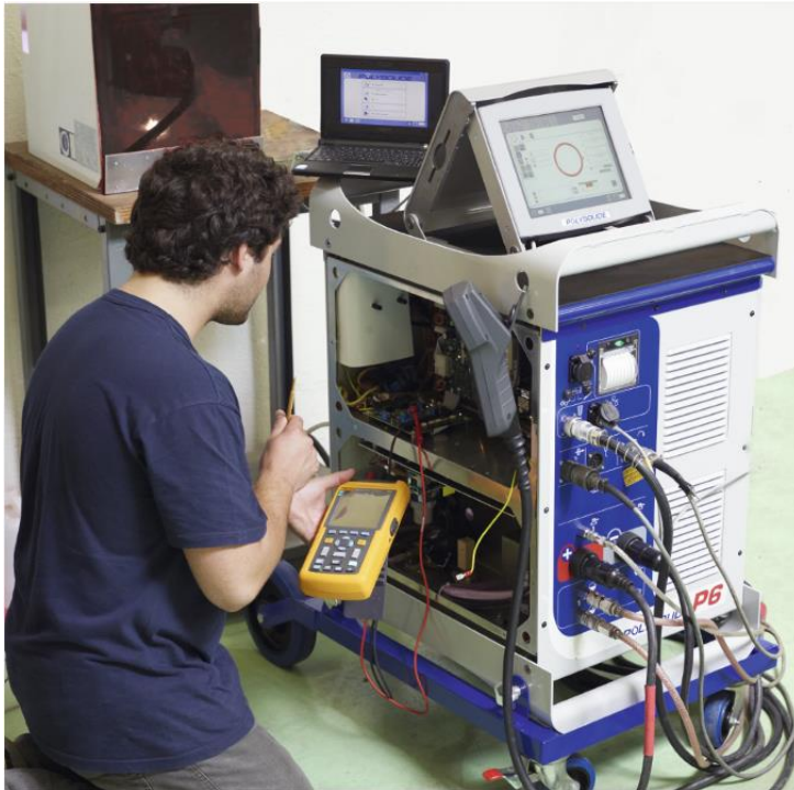
Fig.3 - Measuring and checking a printed circuit board during a maintenance operation on a Polysoude power source
