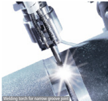
Welding torch for narrow groove joint
