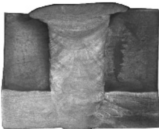
Macrographic section of a narrow groove TIG weld
