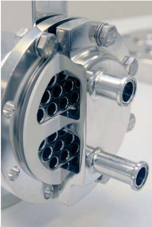
Fig. 4: Aseptic heat exchangers require greater surface quality
