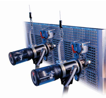
Fig. 9: Several orbital TIG welding heads on duty. A large number of recessed tubes have to be joined to the tubesheet
