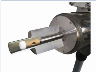
Fig. 11: Longitudinal section of a tubesheet and tube. The orbital TIG welding head is positioned at the front side. The welding lance is introduced into the bore of the tubesheet and partially into the corresponding tube
