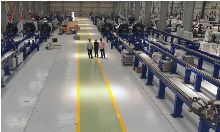
*Fig. 2: Production hall with horizontal 12m TWIN-TIGer rigs*
